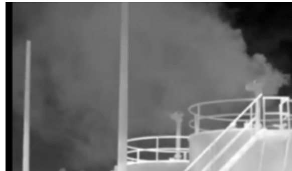
These two images show two hydrocarbon storage tanks in Mexico, at the same moment in time, one viewed with the naked eye, the other viewed with an the infrared FLIR technology. They are emitting methane and deadly volatile organic compounds.
