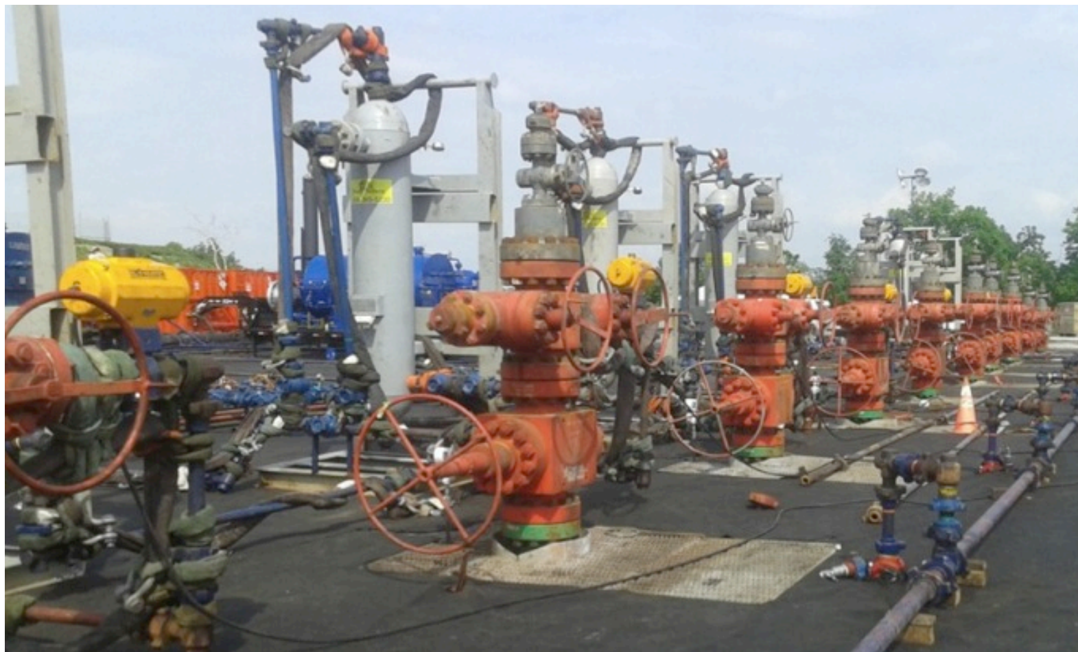
Figure 7: A single well pad may have up to 11 or 12 different wells drills; in this picture the red Christmas tree-like valves close off each well drilled. Ten are visible in the image. Photo: JDTaillant, at a Pennsylvania-Marcellus Shale gas well.
