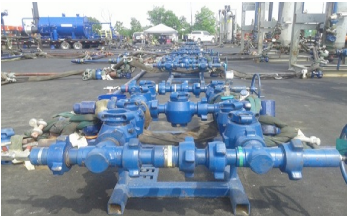
Figure 15: Thousands of joints in fracking pipe unions are potential points of methane leaks. Photo: JDTaillant
