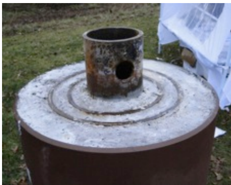
Figure 10: Cemented concentric steel pipe used in fracking wells.
